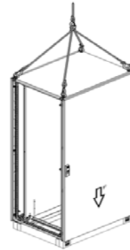
Figure 3-3 Single Section Lifting
